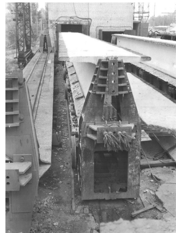
Fig. 1. A prestressed beam on a stand
