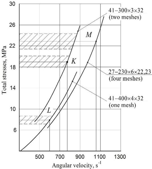
Fig. 4. Dependences of stress change on angular velocity
