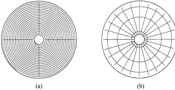
Fig. 2. Wheels reinforcement schemes: (a) tangential and (b) radial
