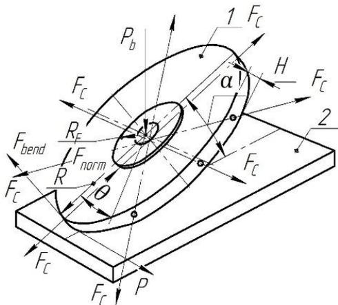
Fig. 1. Forces acting on the cleaning wheel
