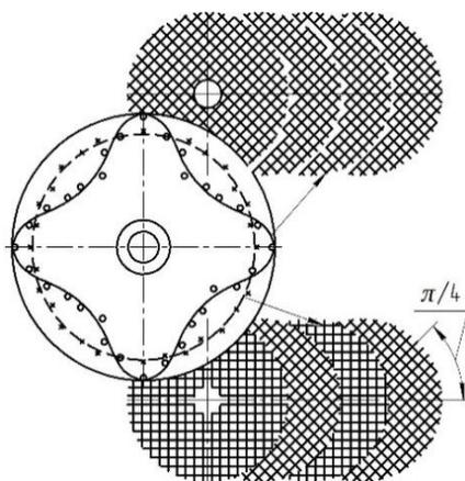
Fig. 3. Diagram of the deformations distribution in the wheel with different orientations of the reinforcing meshes
