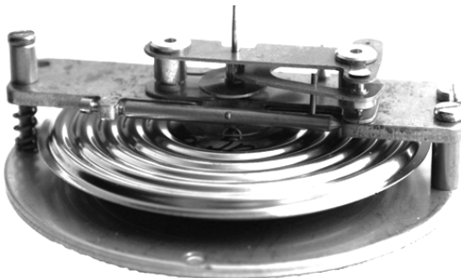
Fig. 6. Corrugated membrane with transmission mechanism
