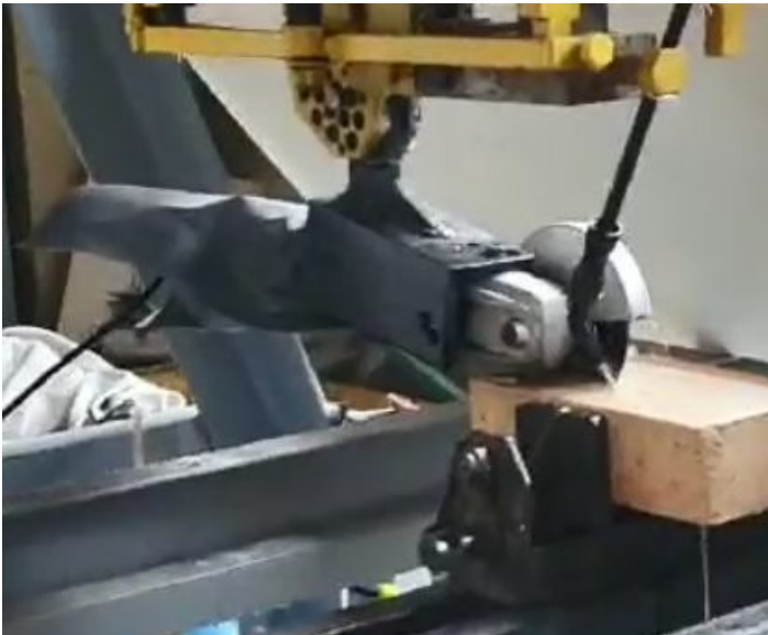
Fig. 3. Cutting refractory bricks on a dynamometric stand
