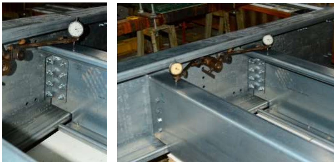
Fig. 1. View of the node of the T-shaped joint of the joint of cold-rolled profiles using a corner and a bolted connection with uncontrolled tension
