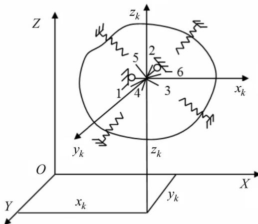
Fig. 2: Stiffness center of vibration damping system
