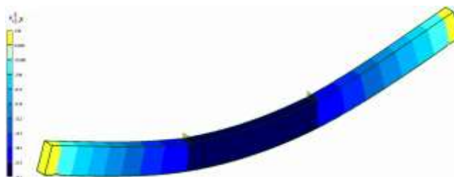
Fig. 15. Displacement mosaic Z(G) (vertical deformations of the model) at maximum loads of 20 kN applied along a single load axis
